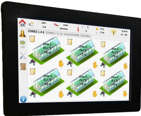
**Fitted with the latest ANJOU AUTOMATION processor, OPTAGROW is a centralised climate, heating and fertilisation-irrigation management computer.**
